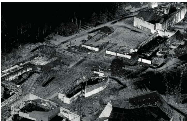
▲ Figure 5, Urban scene mapped with a PLS. The PLS enables collection of complete data from the built environment (e.g. for management and renovation purposes). The operator could use stairs and gateways to reach sections not visible from the street.
