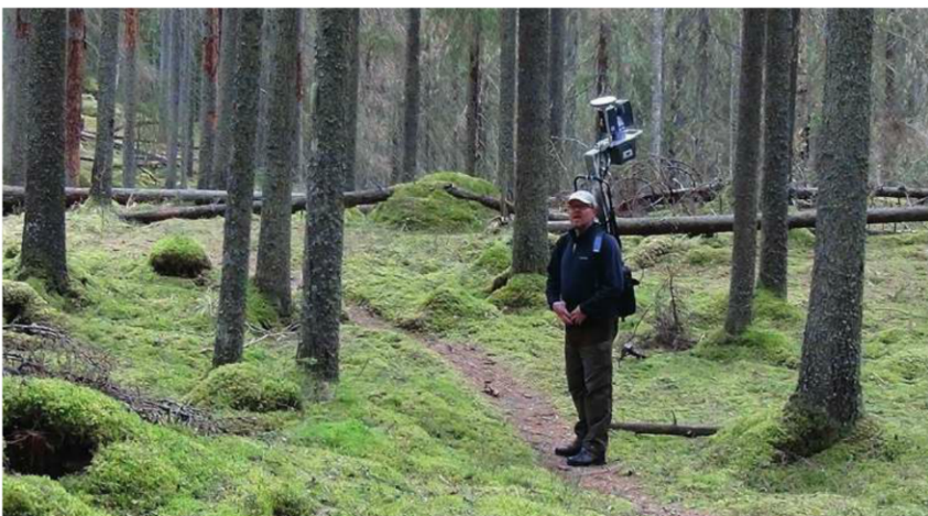
▲ Figure 1, The Akhka R2 PLS system is suitable for detailed mapping of rugged terrain and complex scenes such as forests. The system consists of a laser scanner, GNSS-IMU navigation system, a tablet computer for data recording and a support structure, all carried as a backpack for flexible operation.
